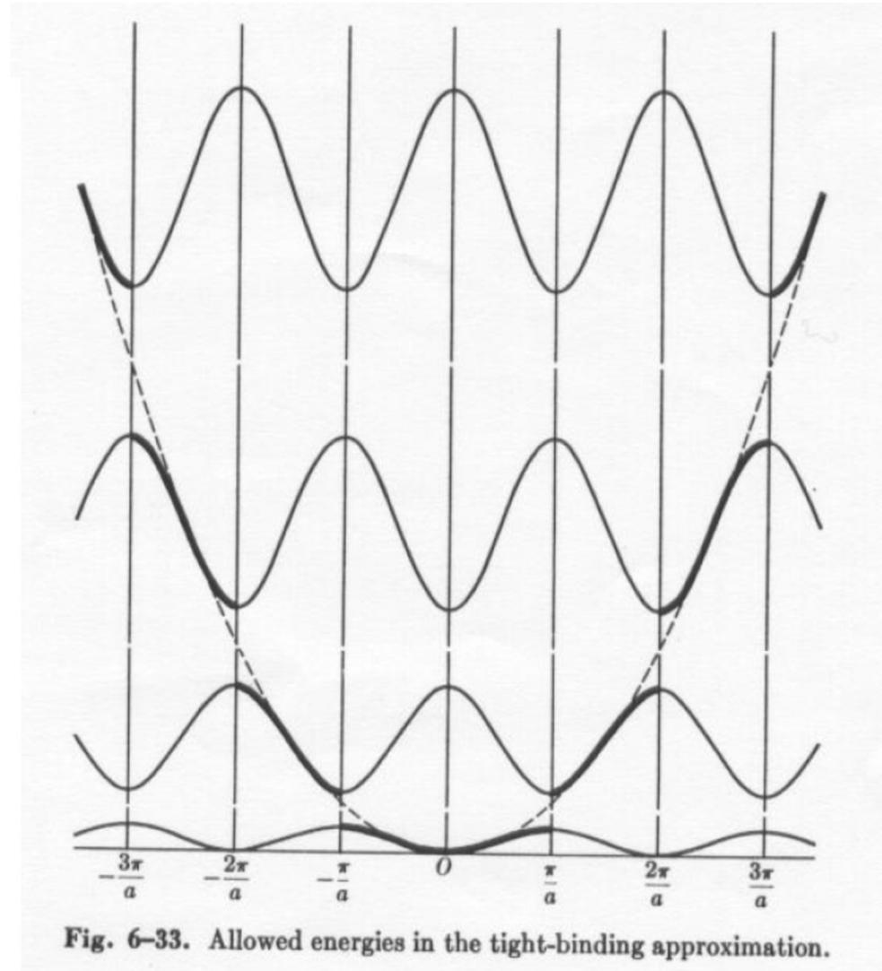
Fig. 6-33. Allowed energies in the tight-binding approximation.
