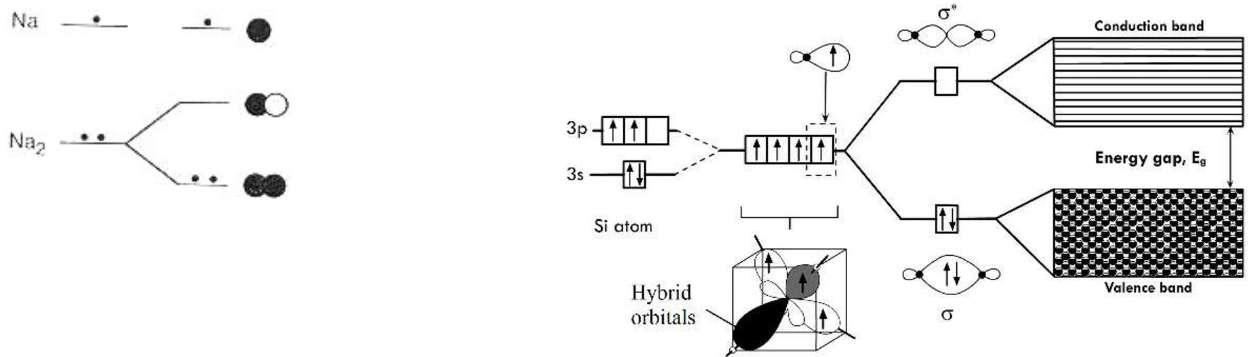
Figure 4: Formation of energy bands in Si. (a) Si atom with 4 electrons in outer shell form (b) 4  $sp^3$  hybrid orbitals. (c) The hybrid orbitals form  $\sigma$  and  $\sigma^*$  orbitals. (d) These orbitals overlap in a solid to form the valence and conduction band. Adapted from *Principles of Electronic Materials* - S.O. Kasap.
