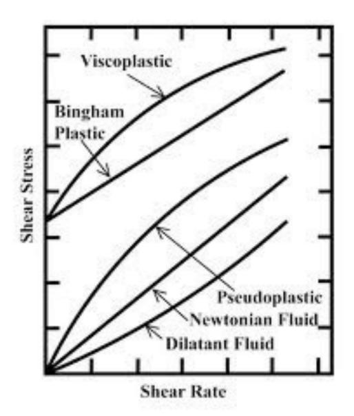
**Shear thinning** is an effect where a fluid's <u>viscosity</u>—the measure of a fluid's resistance to flow decreases with an increasing rate of shear stress. Another name for a shear thinning fluid is a pseudoplastic. This property is found in certain complex solutions, such as lava, ketchup, whipped cream, blood, paint, and nail polish
