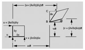
Here  $d\alpha$  and  $d\beta$  are the deformation angles of the figure above,  $d\alpha = CA/CB$
