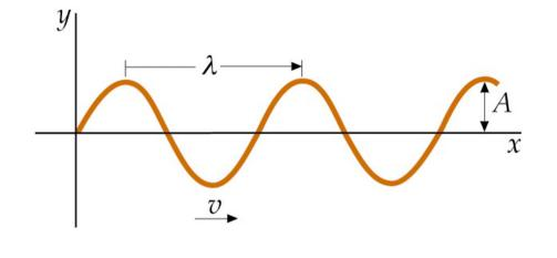
A is the **amplitude** of the wave and  $\lambda$  is the **wavelength** (the distance between two crests); if the wave is moving to the right with speed v, the wavefunction at some t is given by:
