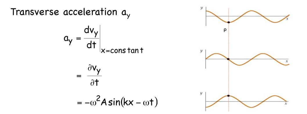
which has a maximum absolute value,  $(a_y)_{max} = \omega^2 A$ , when t=0
