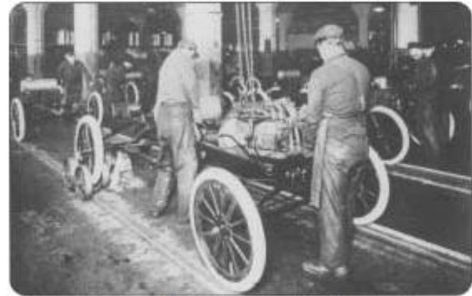
Workers install engines on Model Ts at a Ford Motor Company plant. The photo is from about 1917.
