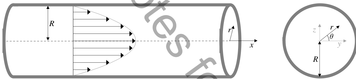
Figure 7.4. Coordinates and flow in a circular vessel.
