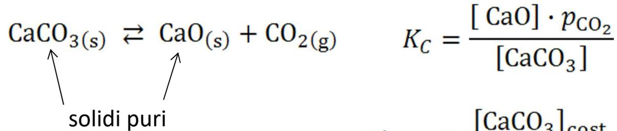
$$K'_C = K_C \frac{[\text{CaCO}_3]_{\text{cost}}}{[\text{CaO}]_{\text{cost}}} = p_{\text{CO}_2}$$
