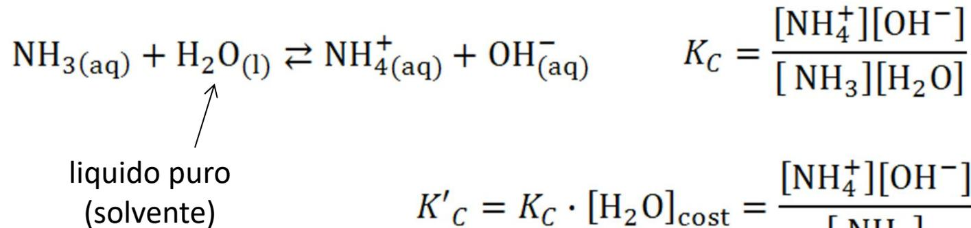
$$K'_C = K_C \cdot [\text{H}_2\text{O}]_{\text{cost}} = \frac{[\text{NH}_4^+][\text{OH}^-]}{[\text{NH}_3]}$$
