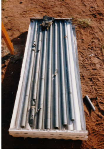
Figure 21: Excellent quality core with very few discontinuities from the massive gneiss of the Rio Grande project in Argentina.
