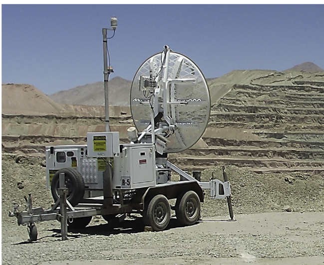
Fig. 27. Radar equipment for monitoring slope displacements.
