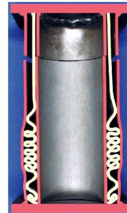
Figure 18: Section through a stress controller showing the buckling inner tube. After Schubert, 1996.
