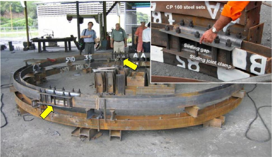
Figure 30. Circular steel arches (W6 X 20) with two sliding joints (detail in inset).
