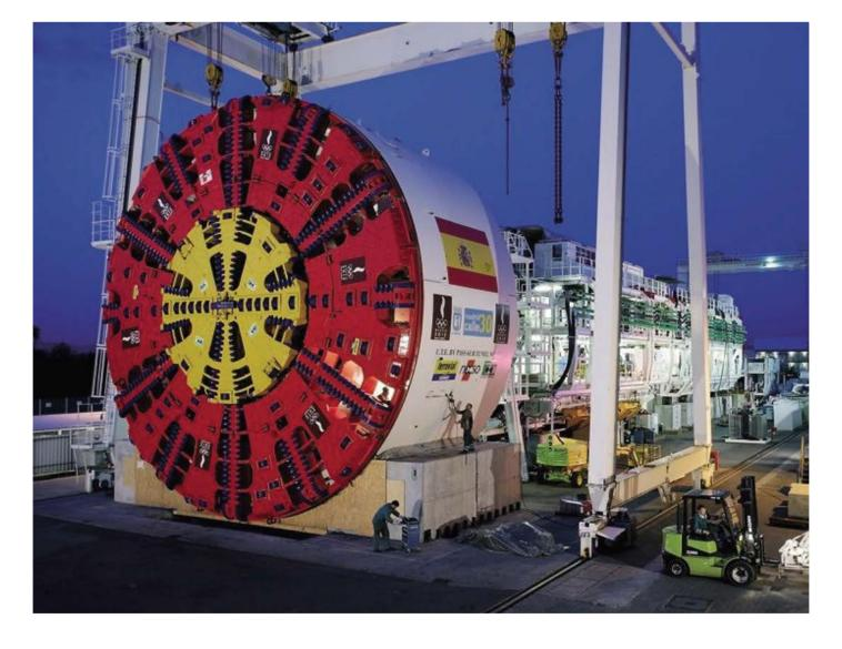
Figure shows the front of the Herrenknecht S-300 EPB TBM used in the construction of the M30-By-Pass Sur Tunel Norte project in Madrid, Spain. The diameter of the cutterhead is almost 50' (15.2 m). See Table D-1 for more data about the machine (Herrenknecht).
