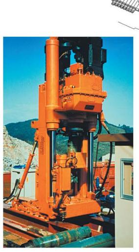
FIGURE 6.2.-64. Shaft excavation by Raise Borer.
