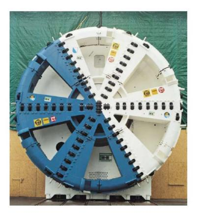
Figure above shows the cutterhead of the Herrenknecht S-256 Single Shield TBM used in the construction of the Islisberg tunnel, Switzerland, which on completion will be the longest underground section of the western Zurich bypass, will be directing transit traffic to central Switzerland around the city. The diameter of the cutterhead is about 38' (11.8 m).
