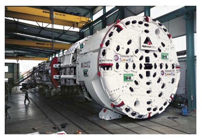
ire D-3 Herrenknecht S-210 Gripper TBM (Herrenknecht)
