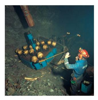
FIGURE 6.2.-63. Cutter used in Raise Boring.
