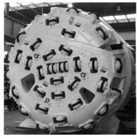
FIGURE 6.2.-55. ATB 50 HA Back loading Cutterhead.
