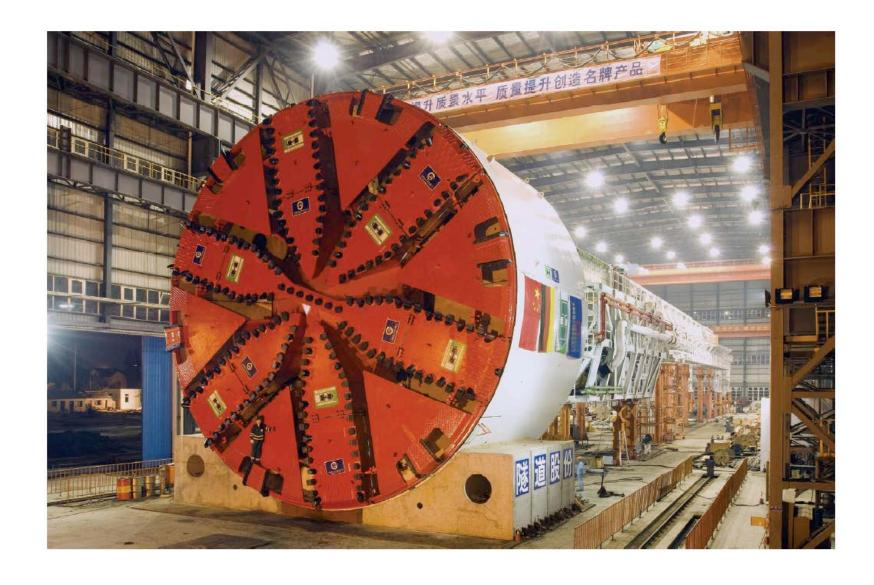
Figure shows the Herrenknecht S-317 Mixshield TBM used in the construction of the Shanghai Changjiang Under River Tunnel Project in China. The diameter of the cutterhead is over 50' (15.4 m).
