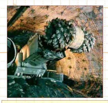
Partial-face machines: use a cutting head on the end of a movable boom (that itself may be track mounted).
