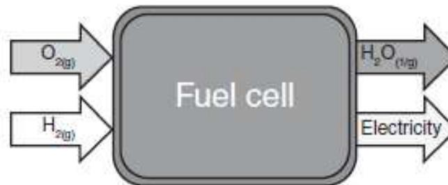
Figure 1.1. General concept of a (H<sub>2</sub>-O<sub>2</sub>) fuel cell.
