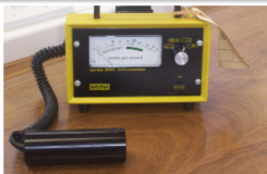
Figure 3.2: How can we find the true count rate of a Geiger counter which suffers from dead-time.
