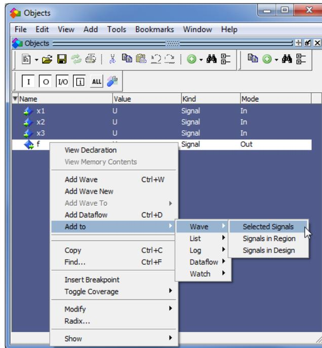
Figure 22. Adding a signal to the Wave window.
