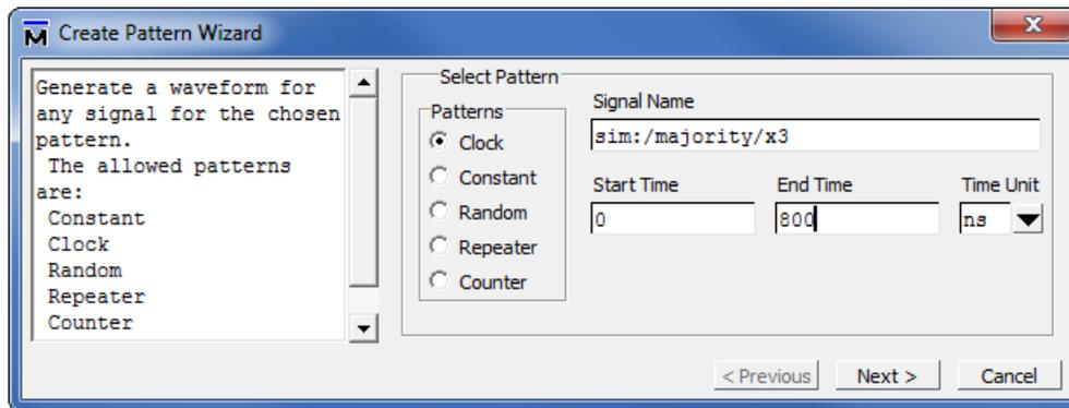
Figure 20. Selecting a signal of clock type.
