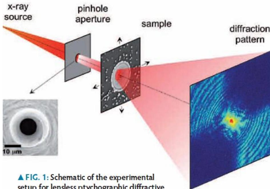
▲ FIG. 1: Schematic of the experimental setup for lensless ptychographic diffractive imaging. The sample is scanned across the x-ray beam defined by a pinhole aperture and for each sample position a diffraction pattern is recorded by a two-dimensional detector.
