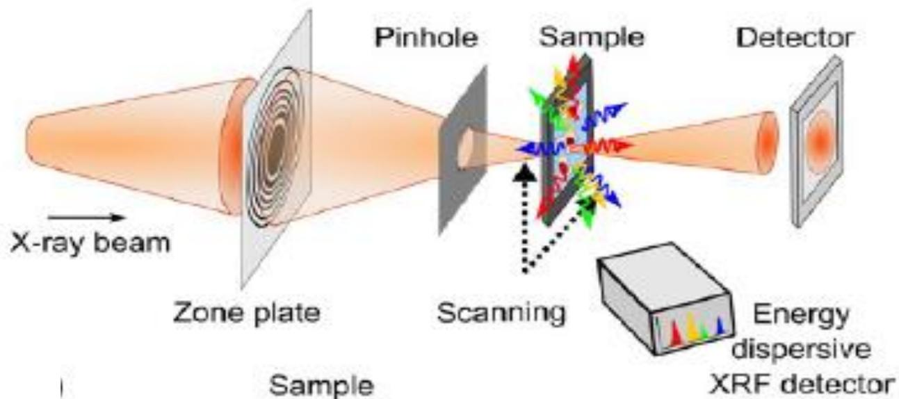
(STXM) with an X-ray fluorescence (XRF) detector
