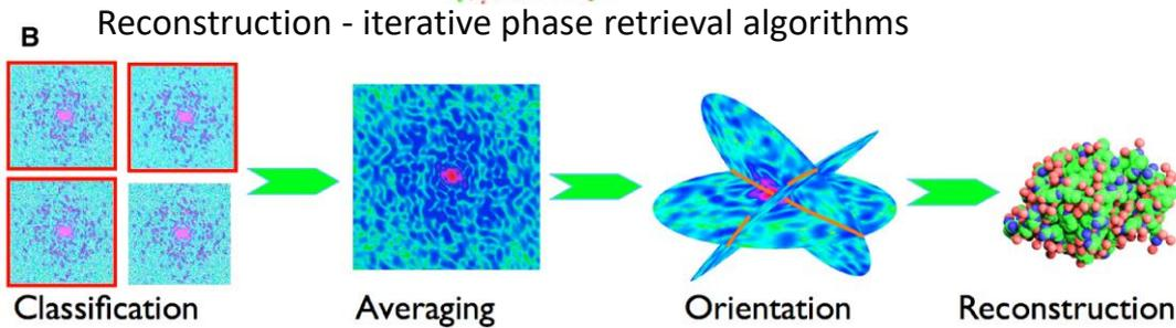
XFEL single-particle diffractive imaging pipeline involves recording single-shot diffraction patterns of the target object before its destruction due to ionization and Coulomb explosion (top), computational purification of single-particle diffraction patterns, orientation determination, classification into 2D class averages, and the 3D merging of intensities in the reciprocal space.
