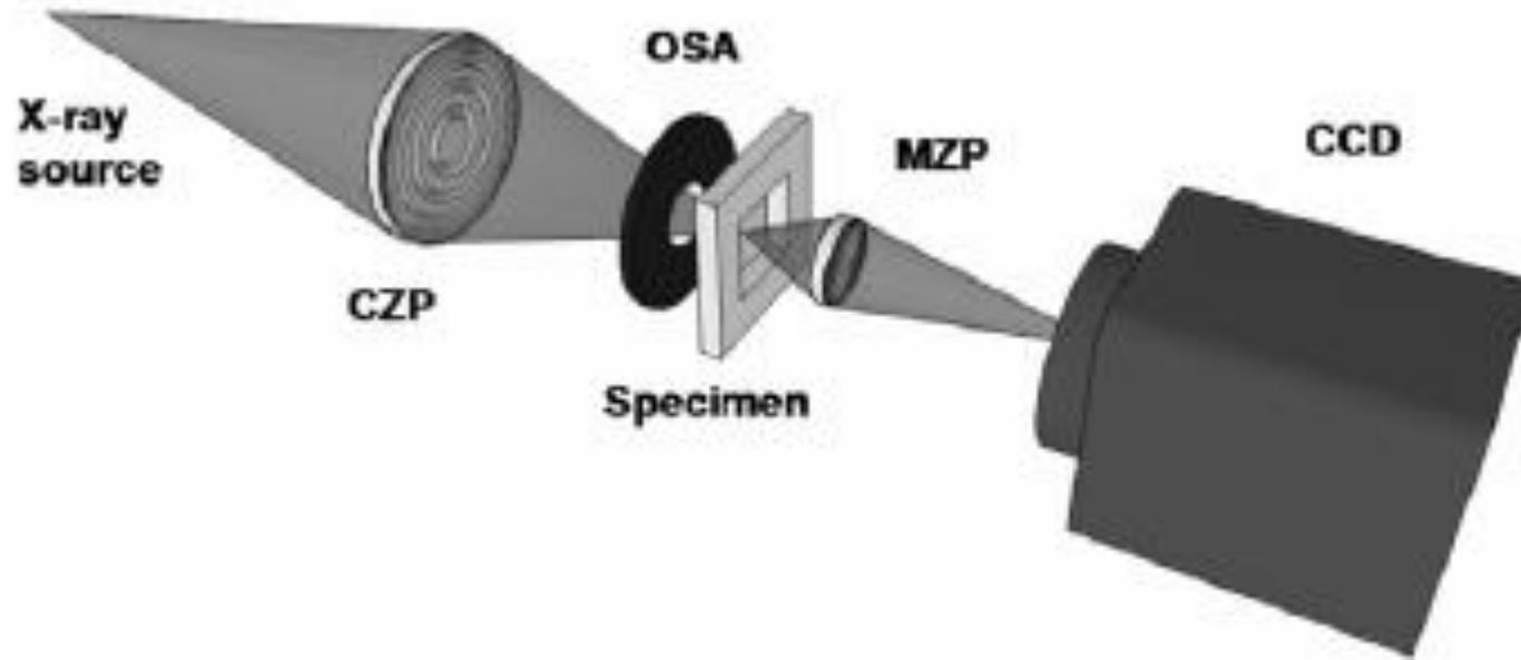
Optical scheme of a full-field imaging microscope (TXM) with x-ray source, condenser zone plate (CZP), specimen, the micro zone plate (MZP) functioning as an objective lens, and a charge-coupled device camera (CCD).
