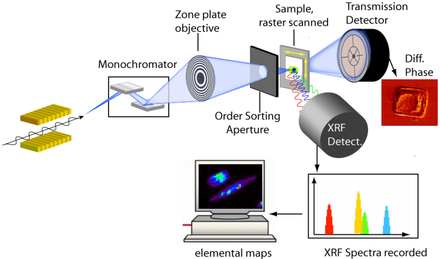
A fluorescence detector can detect (for instance) instance traces of metal in biological systems
