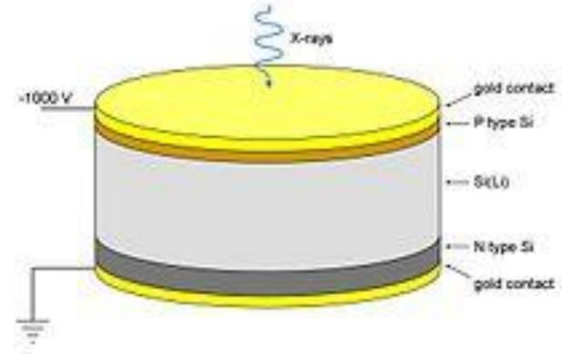
an X-ray photon incident upon the Si(Li) diode will give up its energy to form electron-hole pairs, the number of which is proportional to the energy of the photon
