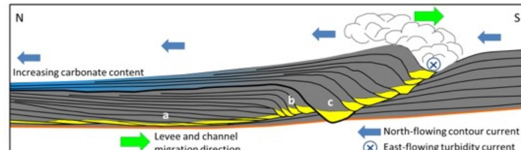
In response to flow-stripping of the suspended load of the turbidity current, the northern levee migrates upstream with respect to contour current, and the channel displaced to the south
