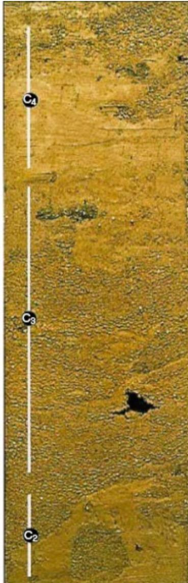
Both positive and negative grading may be present. A mixed siliciclastic–biogenic composition is typical, with evidence of abrasion, fragmented bioclasts and iron-oxide staining.
