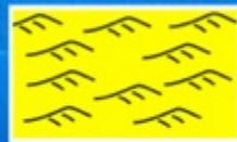
(CFC) M-thick well-sorted fine and very fine sand with large ripples with internal sigmoidal laminae
