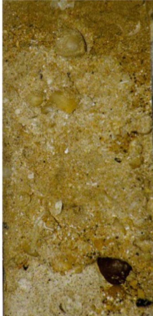
Common in drifts at high latitudes (ice-rafted debris). Under relatively low-velocity currents, IRD remains and is not subsequently reworked. This facies is often indistinguishable from glaciomarine hemipelagites.
