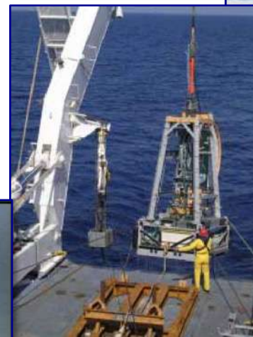
In Situ geotechnical measurements (IFREMER Penfeld Penetrometer)
