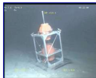
Mid-term temperature/pore pressure lance (SAPPI)
