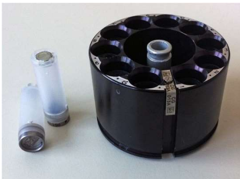
Figure: Carousel suitable for the Sample Changer system present of the XRD1 beamline of Elettra. Each carousel contains up to 10 crystals.
