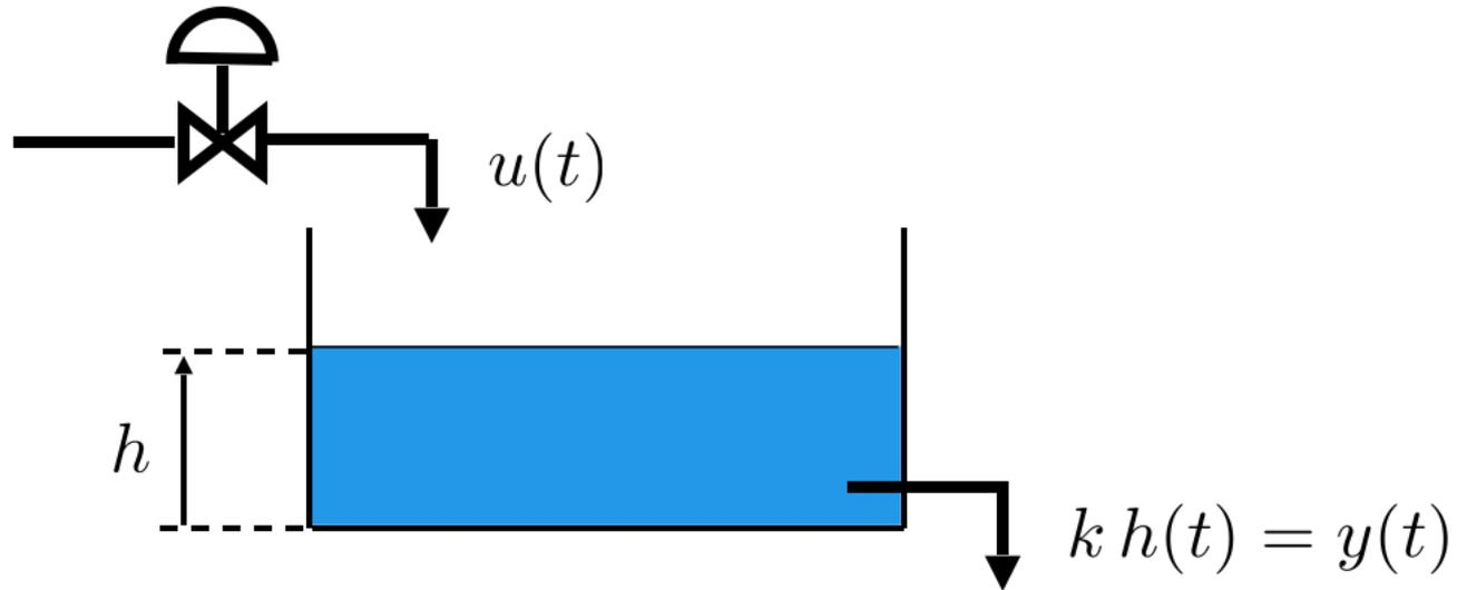
$$\left. \begin{array}{l} u(t), t \in [t_0, t_1] \\ h(t_0) \end{array} \right\} \longrightarrow y(t), t \in [t_0, t_1]$$
