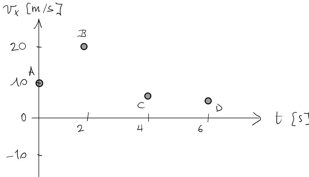
$$\begin{array}{l} A \rightarrow B \\ \left( \begin{array}{l} \Delta t = 2 \text{ s} \\ \Delta v_x = v_{x_B} - v_{x_A} = 20 \text{ m/s} - 10 \text{ m/s} = 10 \text{ m/s} \end{array} \right) \end{array}$$
