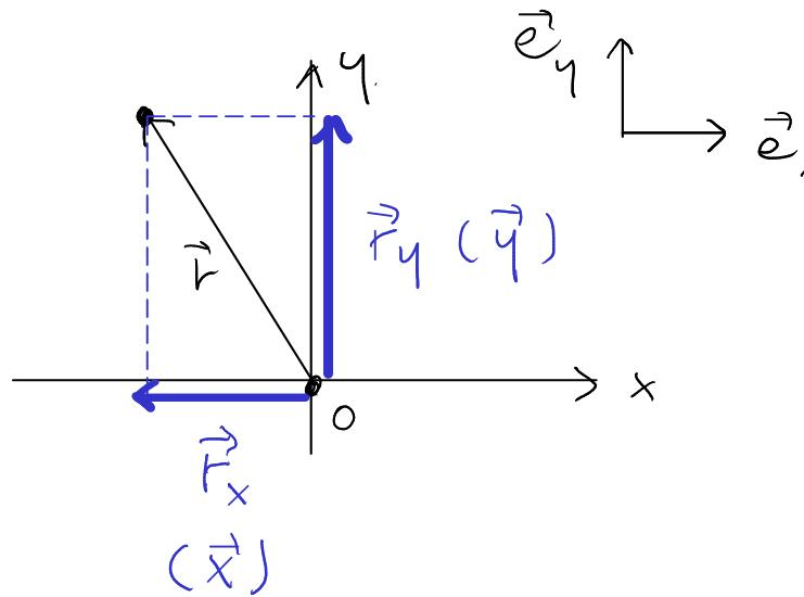
$$\vec{r} = \underbrace{\vec{r}_x + \vec{r}_y}_{\text{vettori componenti}}$$
