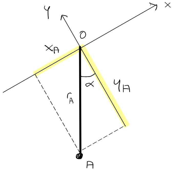
$$\begin{cases} x_A = r_A \cos(90^\circ + \alpha) = -r_A \sin \alpha \\ y_A = r_A \sin(90^\circ + \alpha) = r_A \cos \alpha \end{cases}$$
