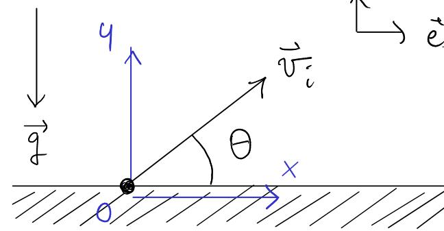
$$\left\{ \begin{array}{l} x = |\vec{v}_i| \cos \theta t \\ y = |\vec{v}_i| \sin \theta t - \frac{1}{2} g t^2 \end{array} \right.$$
