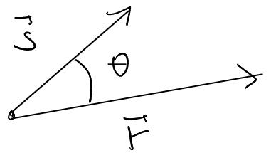
$$\begin{aligned}\vec{r} \cdot \vec{s} &= |\vec{r}| |\vec{s}| \cos \theta \\ &= (r_x \vec{e}_x + r_y \vec{e}_y) \cdot (s_x \vec{e}_x + s_y \vec{e}_y) \\ &= r_x \vec{e}_x \cdot s_x \vec{e}_x + r_y \vec{e}_y \cdot s_y \vec{e}_y \\ &\quad + \cancel{r_x \vec{e}_x \cdot s_y \vec{e}_y} + \cancel{r_y \vec{e}_y \cdot s_x \vec{e}_x}\end{aligned}$$
