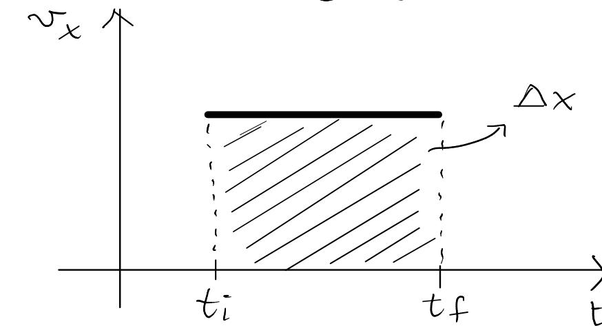
$$\int_{t_i}^{t_f} \underbrace{\frac{dx}{dt}}_{dx} dt = \int_{t_i}^{t_f} v_x dt$$
