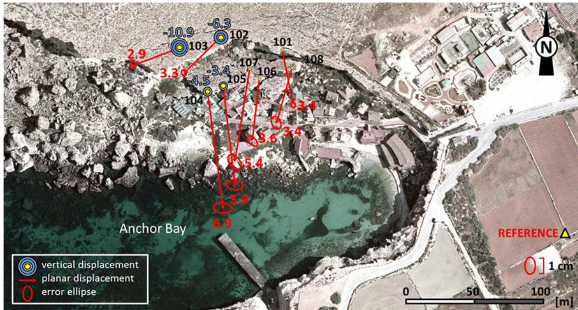
Fig. 8 Cumulated displacement vectors of the GPS network recorded between October 2006 and March 2011 at Il-Prajjet. Benchmarks 101, 102 and 103 are located in the rock spreading area while points 104, 105, 106, 107 and 108 are placed some 15 m below on the block sliding area. Deformation values are expressed in centimetres
