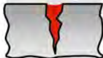
5 Application of developer
