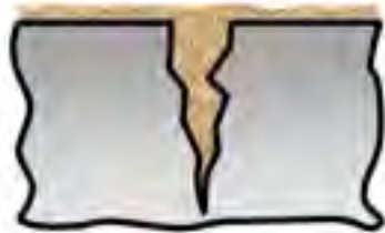
1 Crack filled with dirt
