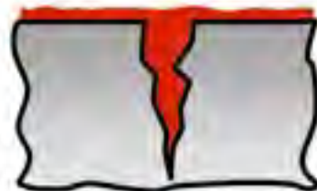
3 Application of penetrant
