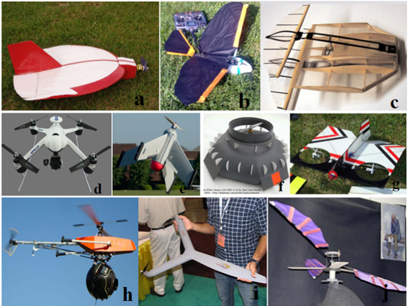
Fig. 5. Different types of MAVs, (a) fixed wing [6], (b) flapping wing [83], (c) fixed/flapping-wing [84], (d) rotary wing [85], (e) VTOL [86], (f) ducted fan [87], (g) tilt-rotor, (h) helicopter [88], (i) unconventional, (j) ornicopter [89].
