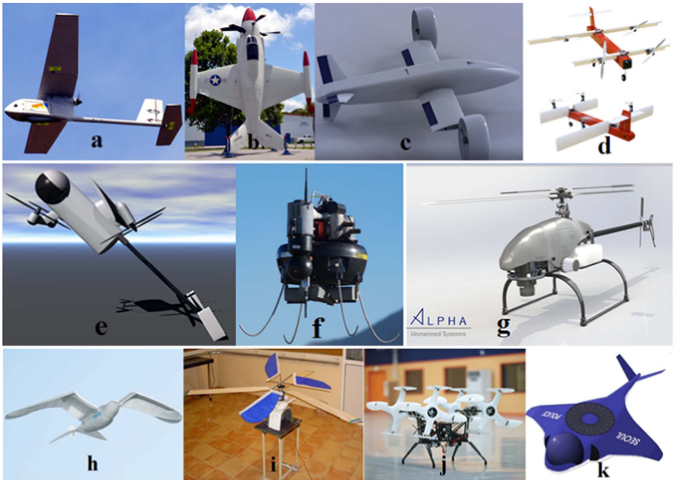
Fig. 4. Different types of \mu UAVs, (a) HTOL [54], (b) VTOL [55], (c) tilt-rotor [56], (d) tilt-wing [57], (e) tilt-body, (f) ducted fan \mu UAV [58], (g) helicopter [59], (h) ornithopter [60], (i) ornicopter [61], (j) cyclocopter [62], and (k) unconventional \mu UAV [63].
