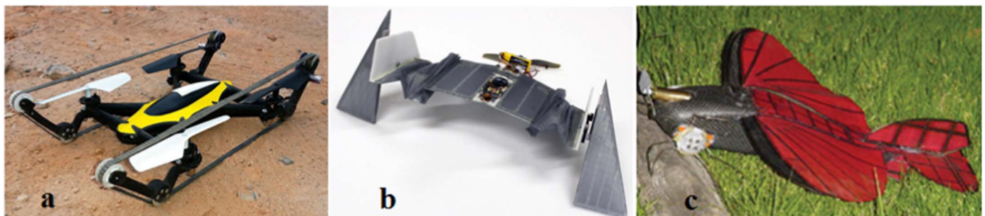
Fig. 13. Air-ground hybrid drones: (a) tank quadcopter [174], (b) DALER robot [175], and (c) MALV [5].
