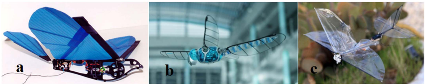
Fig. 6. Different configurations of FWMAVs, (a) monoplane, (b) tandem, and (c) biplane [112].
