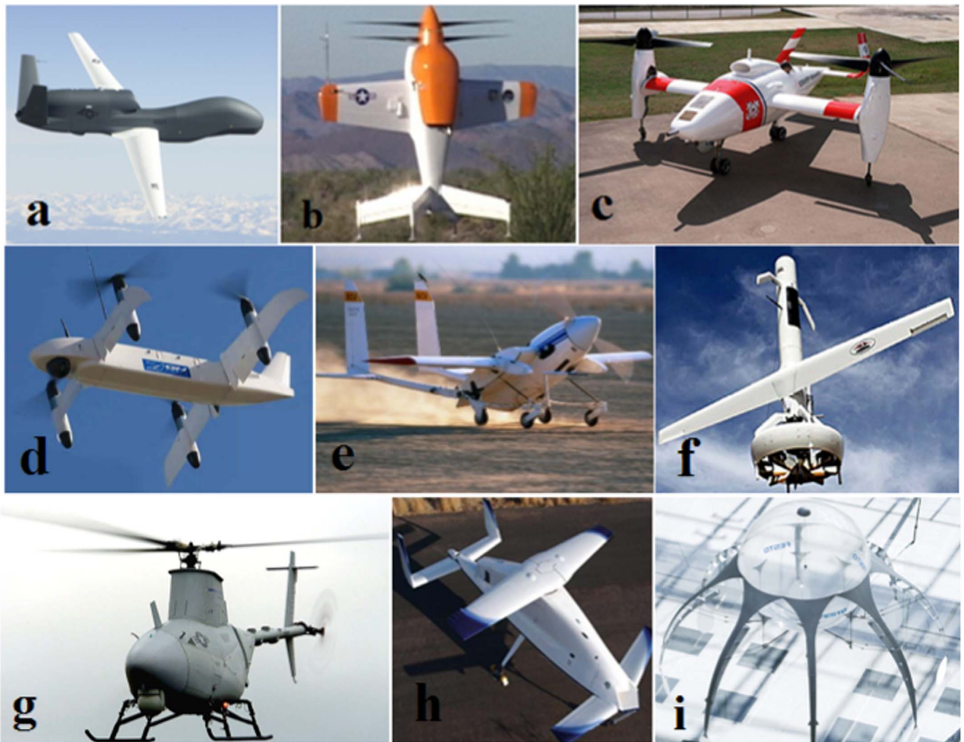
Fig. 3. Different types of UAVs, (a) HTOL [28], (b) VTOL [29], (c) tilt-rotor UAV [30], (d) tilt-wing UAV [31], (e) tilt-body UAV [32], (f) ducted fan UAV [33], (g) helicopter [34], (h) heli-wing [35], and (i) unconventional UAV [36].
