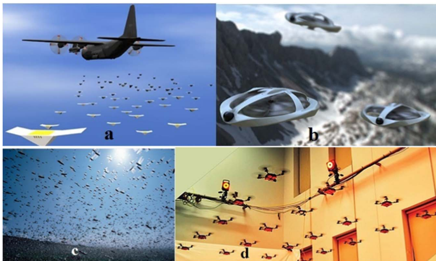
Fig. 31. Swarm flight of (a and b) fixed wing MAVs [399,400], (c) flapping wing PAVs [401], and (d) rotary wings MAVs [402].
