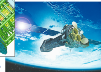
XMM-Newton X-ray telescope: the effects of the radiation environment on its instruments was modeled with Geant4 prior to launch in 1999 (Courtesy of ESA)
