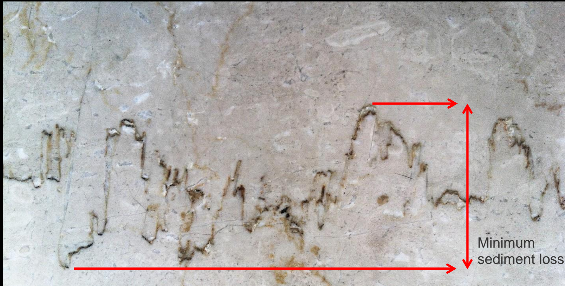
Stylolite from a step on a stair. Most probably from Botticino (Jurassic peritidal carbonates).
