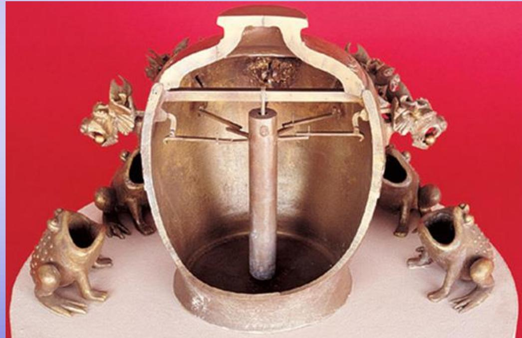
Seismograph designed to detect vertical movement
