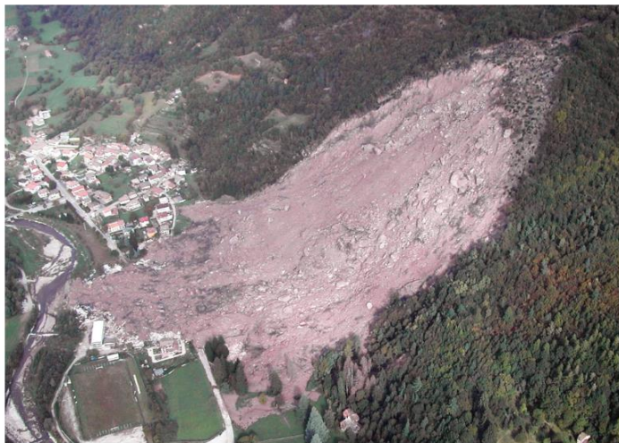
Fig. 12 The 2002 debris avalanche at Cortenova, Lombardy, Italy, which initiated as a translational slide of previously disturbed landslide debris derived from metamorphic rocks (Courtesy of G. Crosta, University of Milan, Bicoca)
