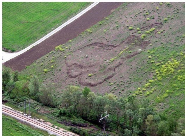
Fig. 37 Shallow planar slide-earthflow, Campania Region, Italy (Photo by O. Hungr)
