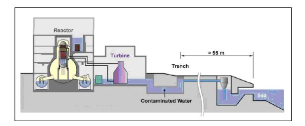
0.1.1 A more interesting illustration is from the TEPCO document, "Result of the Investigation on Tsunami at Fukushima Daiichi Nuclear Power Station" (sic), on the next page. Notice that the doors to both the reactor building and the turbine building are shown as inundated. The caption for the illustration is taken directly from the report.
