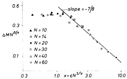
FIG. 17. Finite-size scaling plot for the correction to the bulk finite-size order-parameter behavior for lattices with free edges.  $\Delta M = M - B\epsilon^{1/8}$ , with  $B = 1.22$ . The solid line is the best fit assuming the asymptotic scaling form  $B_s x^{\beta_s}$ , with  $\beta_s = \beta - \nu = -7/8$ , and yields  $B_s = 0.60$ .
