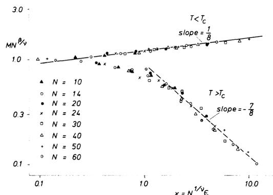
FIG. 14. Finite-size scaling plot for the order parameter for lattices with p.b.c. Data for  $N=10$ ,  $\blacktriangle$ ;  $N=14$ ,  $\circ$ ;  $N=20$ ,  $\bullet$ ;  $N=24$ ,  $\times$ ;  $N=30$ ,  $\square$ ;  $N=40$ ,  $\triangle$ ;  $N=50$ ,  $+$ ;  $N=60$ ,  $\odot$ . For  $T < T_c$  the solid line is  $1.22 x^{1/8}$ ; for  $T > T_c$  the dashed line is  $0.92 x^{-7/8}$ .
