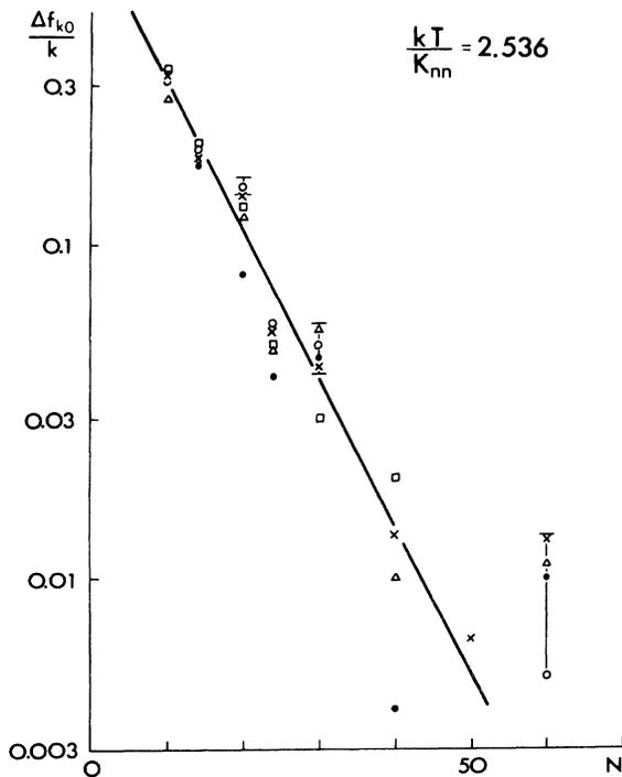
FIG. 11. Variation of  $\ln(\Delta f/k)$  vs  $N$ , where  $\Delta f = f_{k0}(N) - f_{k0}(\infty)$  for  $kT/K_{nn} = 2.536$ . The solid line is the best fit with slope equal to 0.104 and  $k = 2, \circ$ ;  $k = 3, \times$ ;  $k = 4, \triangle$ ;  $k = 6, \bullet$ .
