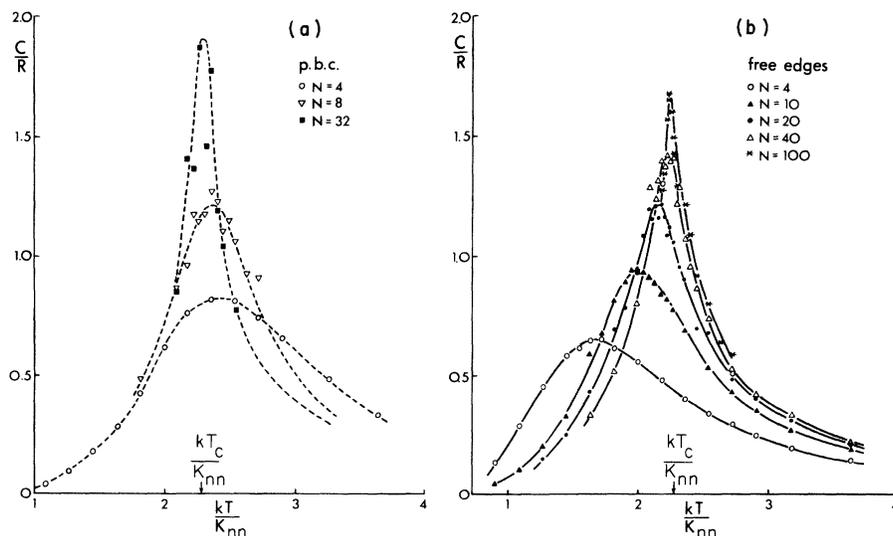
FIG. 3. Temperature dependence of the specific heat. The dashed curves in (a) are the exact curves of Ferdinand and Fisher (Ref. 3).  $kT_c(\infty)/K_m = 2.269$ .
