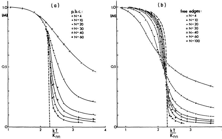
FIG. 4. Temperature variation of the order parameter. The dashed lines represent the exact  $N=\infty$  curve (Ref. 1).
