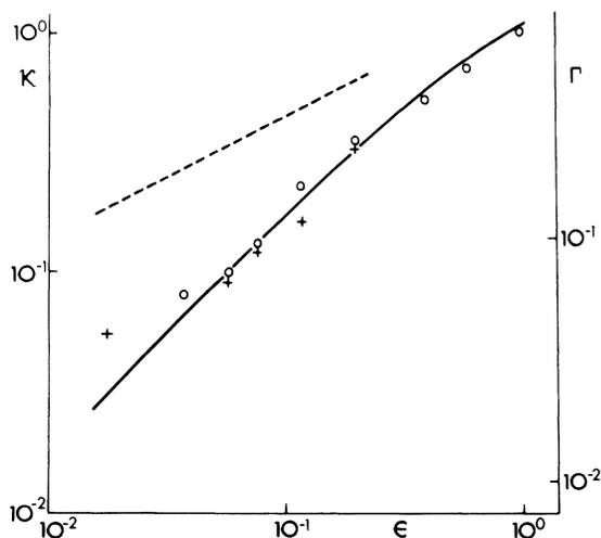
FIG. 13. Variation of  $\kappa(T)$  and  $\Gamma(T)$  vs  $\epsilon$ . The scale on the left-hand side is for  $\kappa(\circ)$  and the scale on the right-hand side is for  $\Gamma(+)$ . Actual  $N=\infty$  variation of  $\kappa$ , —; Bethe approximation for  $\kappa$ , --- (see Ref. 28).
