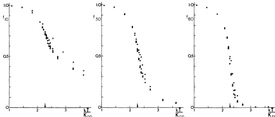
FIG. 7. Temperature variation of spin-spin correlation functions for  $N \times N$  lattices with p.b.c.  $f_{k0}$ :  $N = 4$ ,  $\circ$ ;  $N = 10$ ,  $\blacktriangle$ ;  $N = 20$ ,  $\bullet$ ;  $N = 40$ ,  $\triangle$ ;  $N = 60$ ,  $\circ$ . The arrows show  $T_c(\infty)$ .
