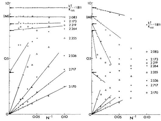
FIG. 9. Linear extrapolation of the order-parameter data to  $N = \infty$ : p.b.c. data to the left-hand side, free-edge data to the right-hand side. The arrows give exact infinite-lattice values (see Ref. 1).  $kT_c(\infty)/K_{nn} = 2.269$ .
