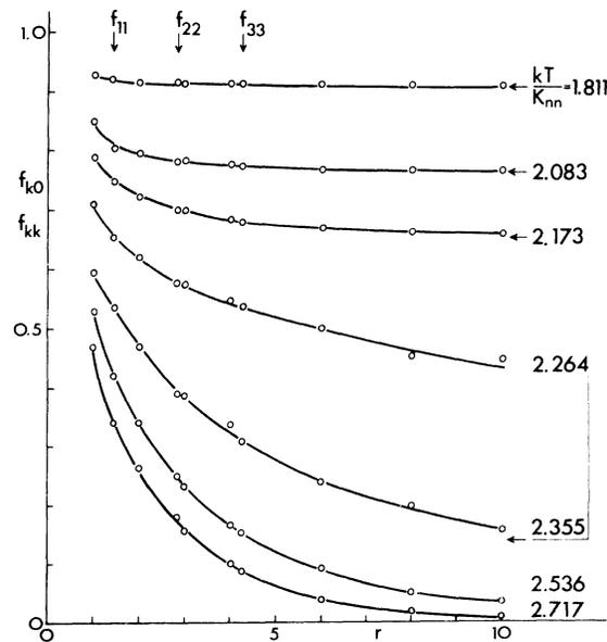
FIG. 12. Variation of row and diagonal spin-spin correlations with  $r$ . The circles are the extrapolated  $N = \infty$  values. The arrows on the right-hand side give  $M^2(T)$ .
