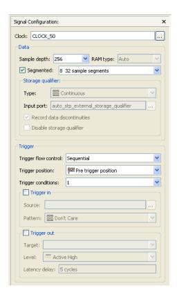
Figure 16. Select Segmented buffer acquisition mode with 8 32 sample segments.
