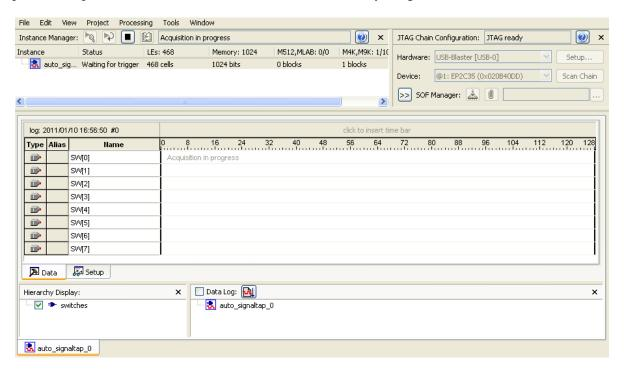
Figure 11. SignalTap II window on a DE-series board after Run Analysis has been clicked.
