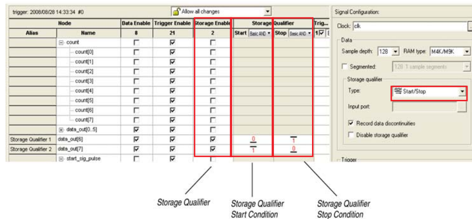
Figure 13-16. Start/Stop Mode Storage Qualifier Setup
