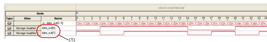
Figure 13-14. Data Acquisition of a Recurring Data Pattern in Continuous Capture Mode (to illustrate Conditional capture)
