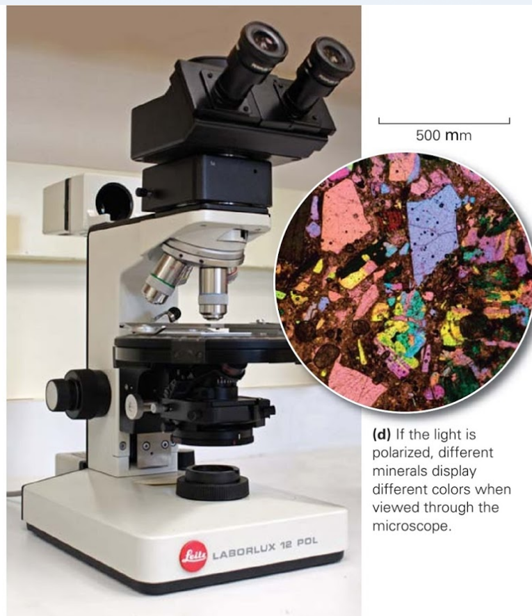
(c) With a petrographic microscope, it's possible to view thin sections with light that shines through the sample from below.
