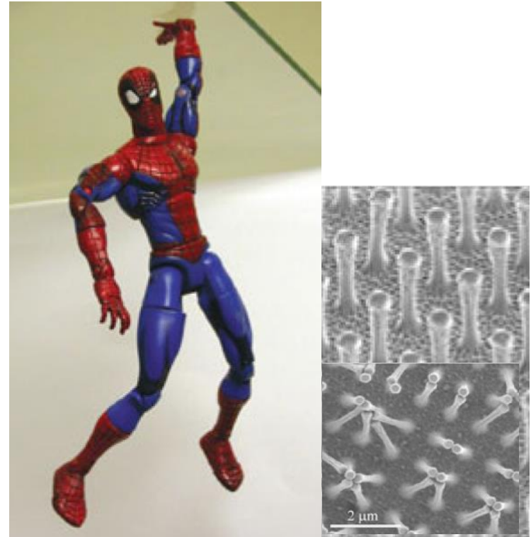
Polyimide pillars (before and after use)
