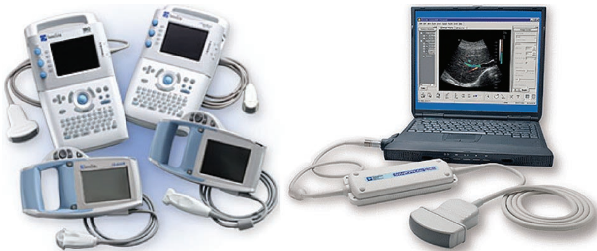
Figure 21. Photographs show commercially available small US scanners from two vendors. (a) The upper scanners are 13.3 in (33.8 cm) tall and weigh 5.7 lb (2.6 kg), whereas the lower scanners weigh about 3 lb (1.4 kg). (b) The dedicated electronics module attached to the transducer cable weighs 10 oz (0.3 kg) and is 7.6 in (19.3 cm) long. (Fig 21a courtesy of SonoSite, Bothell, Wash; Fig 21b courtesy of Terason, Burlington, Mass.)
