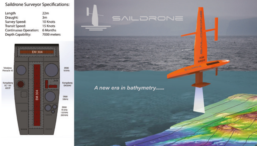
FIGURE 8.4 Autonomous Saildrone equipped with deep water multibeam mapping system
