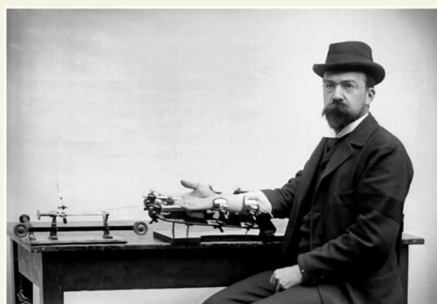
Figure 7 Angelo Mosso performing one of his experiments. Here Mosso is photographed with his pneumograph at pneumatic transduction with two drums, an evolution of Marey's pneumograph, which in contrast had only one drum with a flexible guttapercha membrane (courtesy of Marco R. Galloni).
