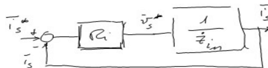
$$\frac{\bar{v}_s - \frac{\bar{i}_s}{\bar{i}_s}}{1 + \frac{R_i}{z_{in}}} = \frac{1}{1 + \frac{z_{in}}{R_i}}$$
