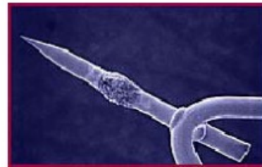
Single oriented W crystal fine tip
