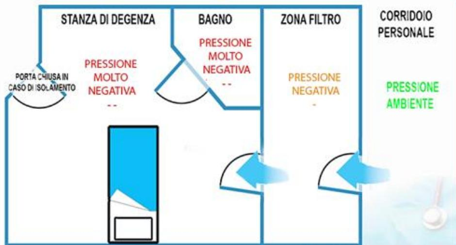
IL SISTEMA DI PRESSIONI TIENE I MICROORGANISMI PATOGENI DENTRO LA STANZA DI DEGENZA. PERCHÉ IL SISTEMA FUNZIONI, PRIMA DI APRIRE LA PORTA INTERNA, QUELLA ESTERNA DEV'ESSERE CHIUSA, E VICEVERSA.
