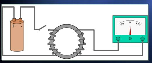
A Faraday's iron ring apparatus: Change in the magnetic flux of the left coil induces a current in the right coil
