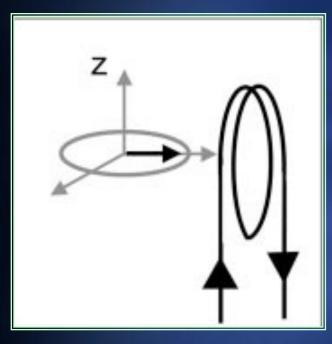
Coil is both transmitter and receiver
