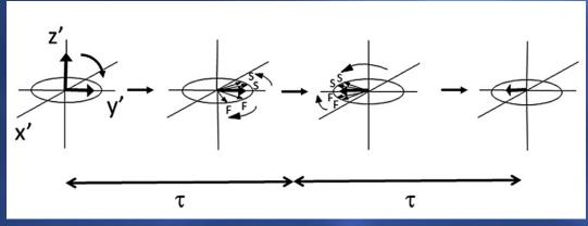
The 'fan' of isochromats is 'flipped' to the other side of the transverse plane
