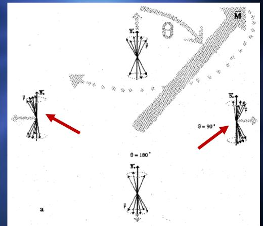
T<sub>1</sub> Quantum mechanics If the quantum of energy is lost from the spin system, there is an increase in the population of the higher energy level  $\checkmark$  resulting in an increase in M<sub>7</sub> T<sub>1</sub> relaxation the emitted quantum of energy is absorbed by the surrounding environment • known as the lattice
