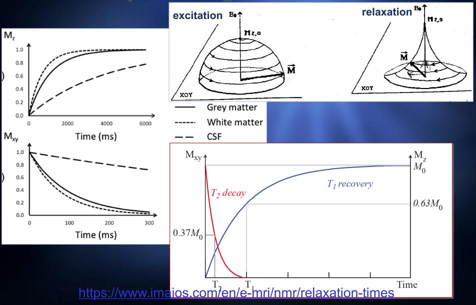
Relaxation and quantum mechanics nutation of the M results from absorption of energy from the RF field
