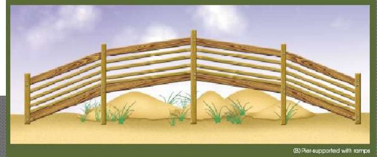
(B) Pier-supported with ramps
