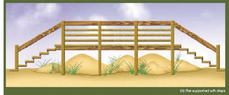
(A) Pier-supported with steps
