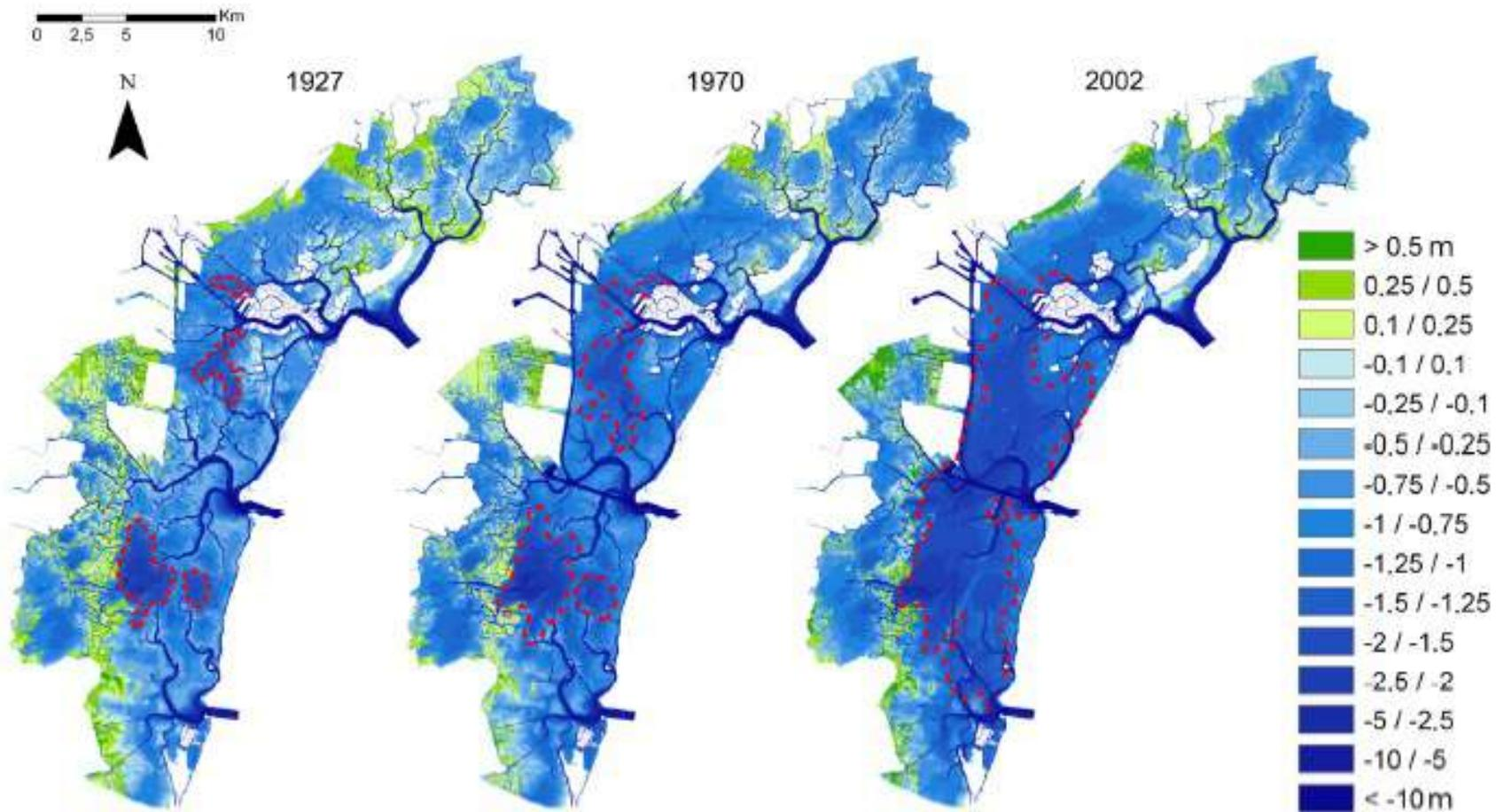
Fig. 3. Colour-shaded bathymetric maps of Lagoon of Venice (from left to right: 1927, 1970; 2002). Dotted red line indicates migration of  $-1.2\text{m}$  contour line, showing an overall increase in depth (progressively darker blue colour). Emergent areas are indicated in green. (For interpretation of the references to colour in this figure legend, the reader is referred to the web version of this article.)
