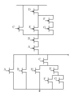
$$Y = \overline{A} \cdot \overline{B} + \overline{CD} = \overline{(A+B) \cdot CD}.$$
