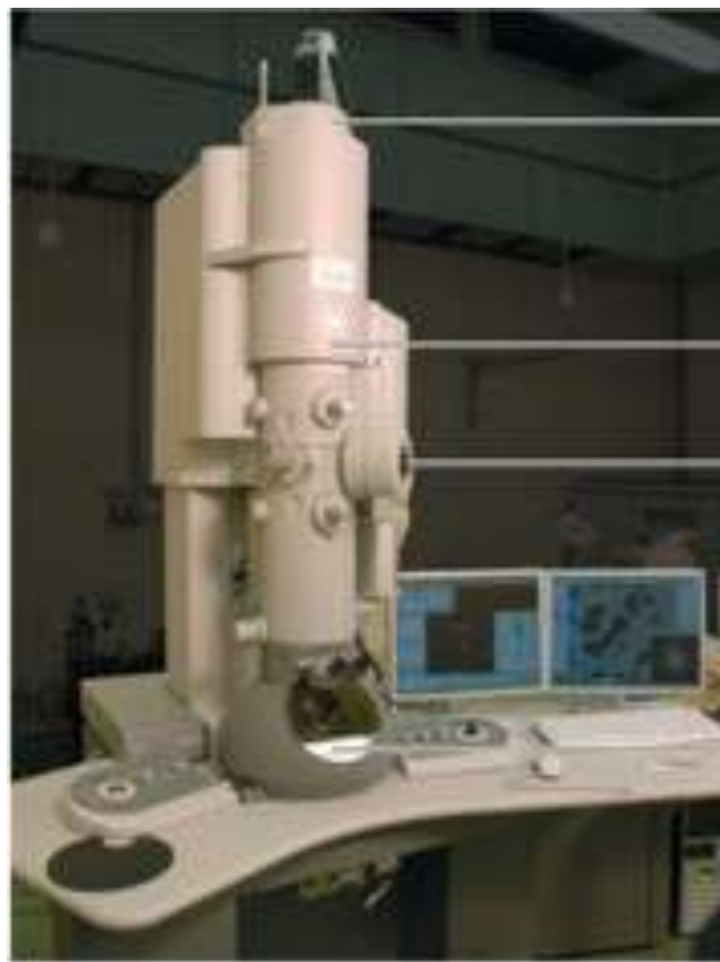
Figure 1.23 The electron microscope. This instrument encompasses both transmission and scanning electron microscope functions.
