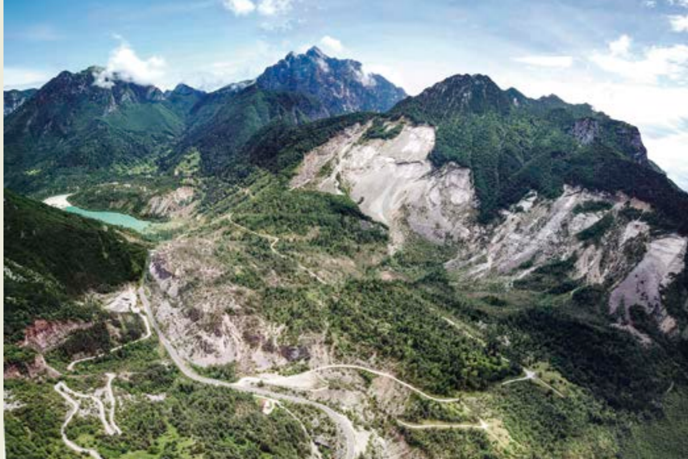
The extensive scarp and the huge body of the Vajont landslide detached from Mt. Toc. (Drone photo courtesy Monica Ghirotti).
