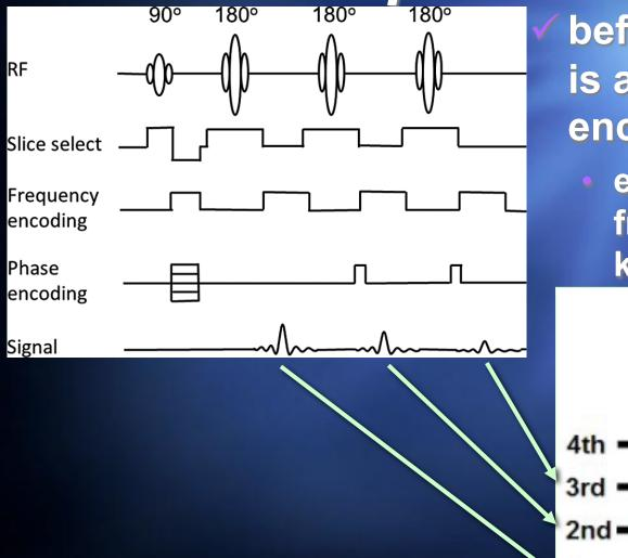
before each echo there is an additional phase encoding gradient
