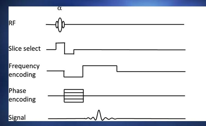
It the refocusing pulse is omitted the echo is generated only by switching of gradients on the frequency encoding axis
