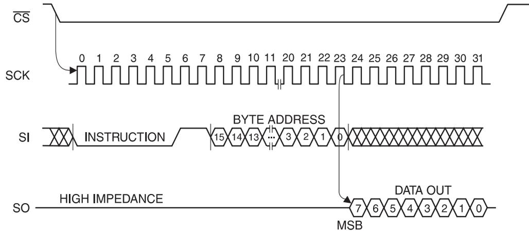
Figure 9. WRITE Timing
