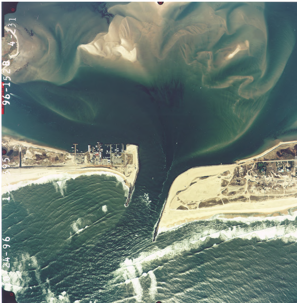
Figure IV-3-29. Shinnecock Inlet, New York, 24 October 1996. The inlet has been stabilized with stone jetties 800 ft apart. The beach east of the inlet has advanced to the end of the east jetty. To the west, the shore has suffered chronic erosion, requiring frequent emergency repair by the highway department to prevent the road from being breached. The ebb shoal (only partially shown in this photograph) is an unsymmetric oval that attaches to the downdrift beach about 1,200 m west of the west jetty (Photograph courtesy of USAED, New York)
