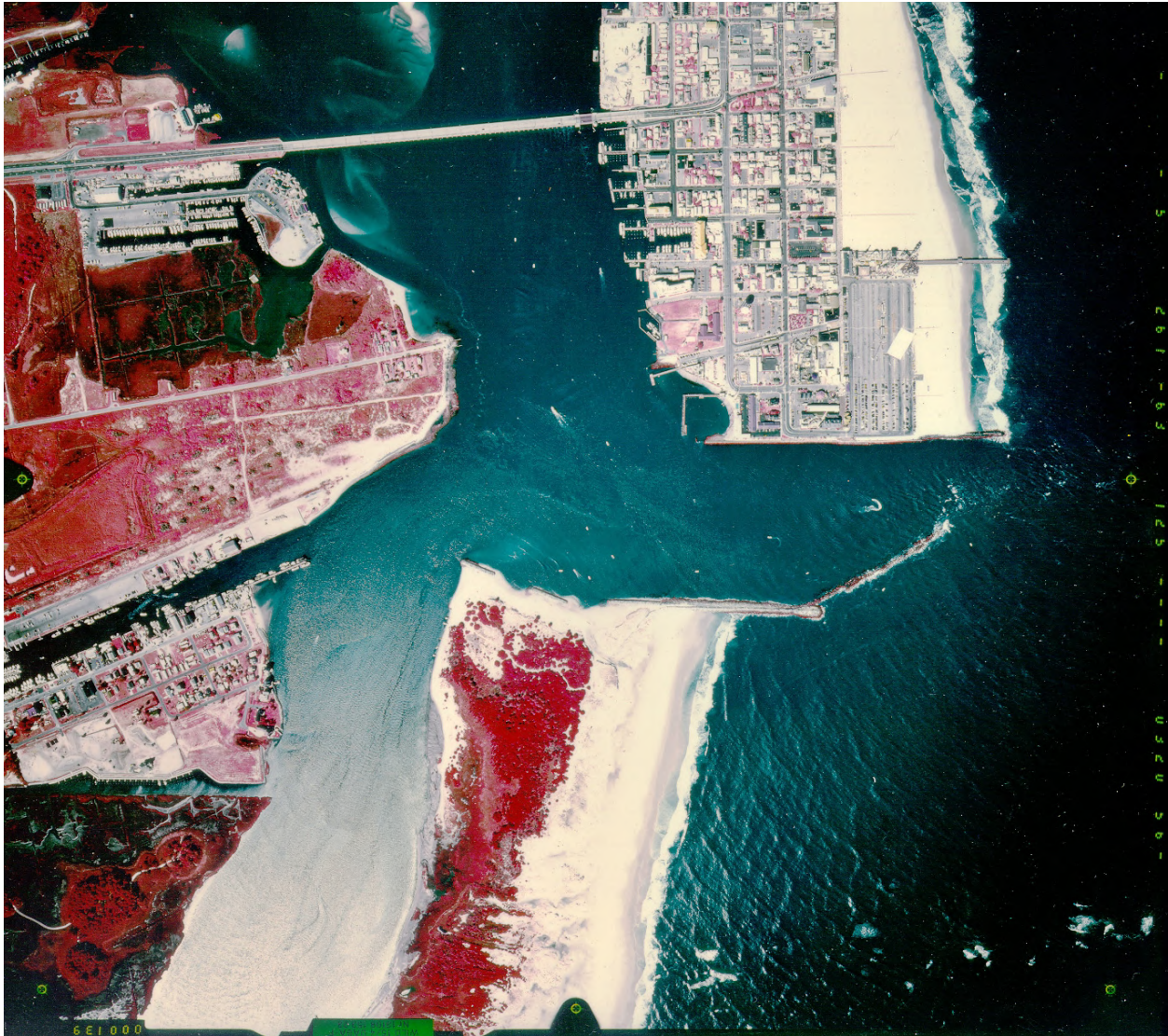
Figure IV-3-21. Ocean City Inlet, Maryland, 11 September 1995. Before the 1933 hurricane breached the barrier island, Assateague and Fenwick Islands were joined and had a straight shoreline. The former shoreline ran approximately along the seaward-most road (Photograph provided by USAE District, Baltimore)
