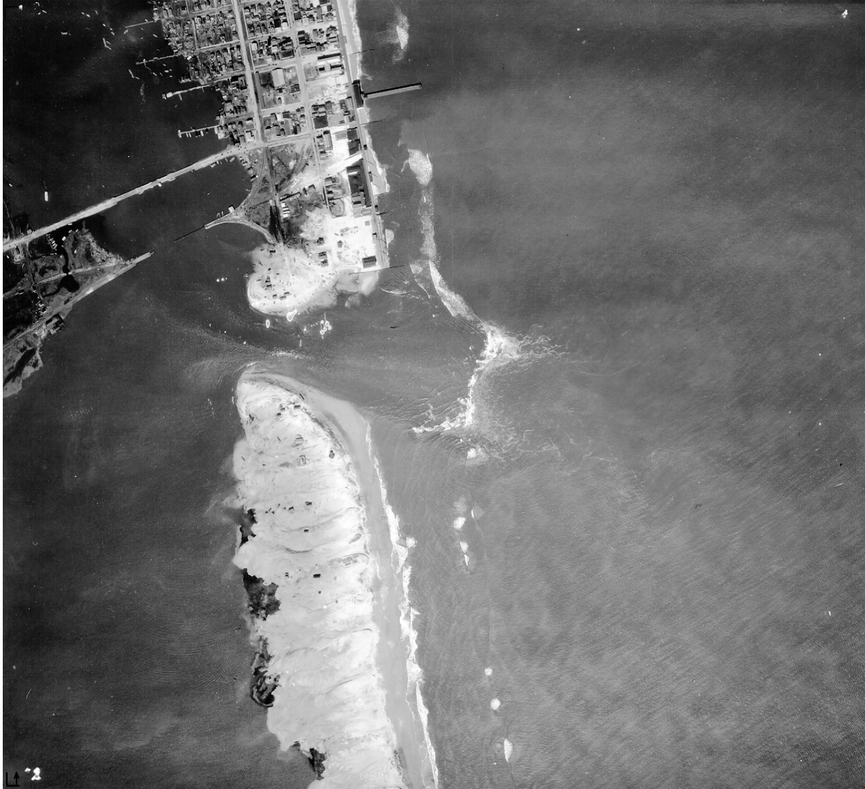
Figure IV-3-20. Ocean City Inlet, Maryland, September 1933. Ocean City is on Fenwick Island in the top center of the image, the Atlantic Ocean is to the right, and Assateague Island is on the bottom. This photograph was taken only one month after a hurricane breached the barrier island. Note waves breaking at the edge of a small ebb shoal. (Photograph from Beach Erosion Board archives)
