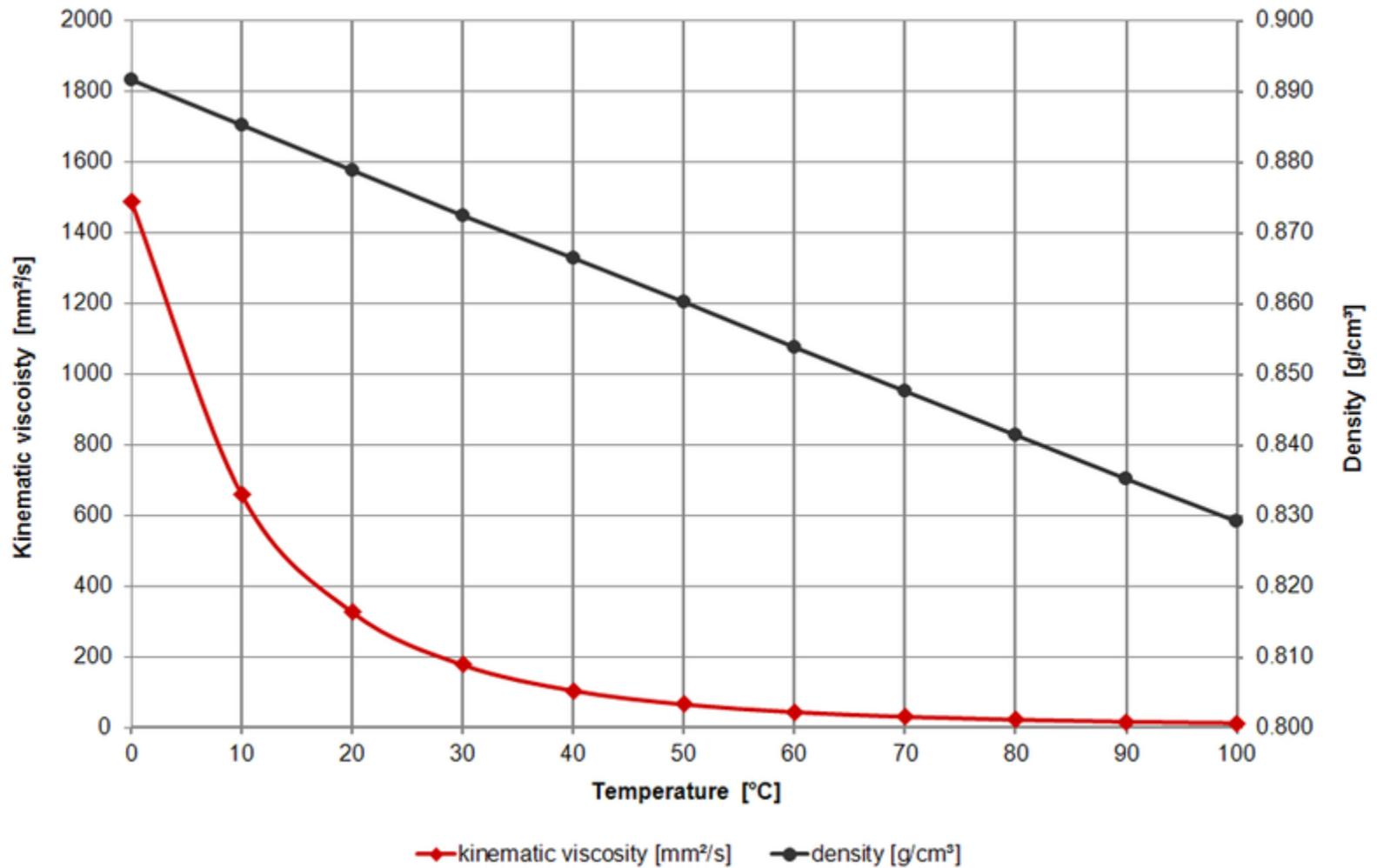
Engine Oil SAE 15W-40 - kinematic viscosity and density over temperature
