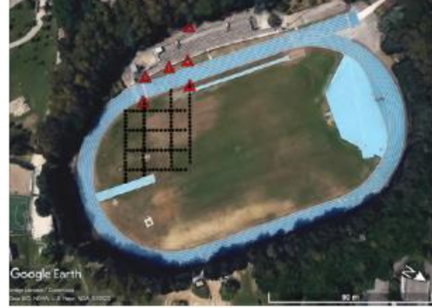
Figure 4.1: (a) Location of Matera test site (blue square) and the epicenter of the M4.6 Catanzaro earthquake on 25.10.2019 (red star). (b) Satellite view of Matera test site. Athletic field instrumentation deployment is indicated with red triangles (three-component sensors) and black dots (vertical geophones).
